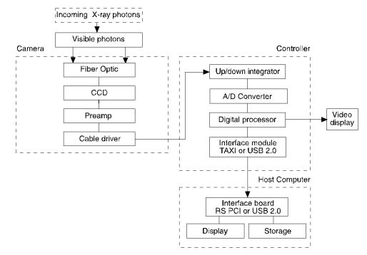
Figure 8. Block Diagram of Signal Path in System
